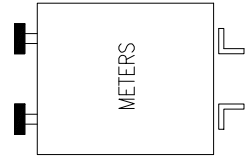
ANGLE BRACKETS 50x50mm FOR NON DOMESTIC METERS
